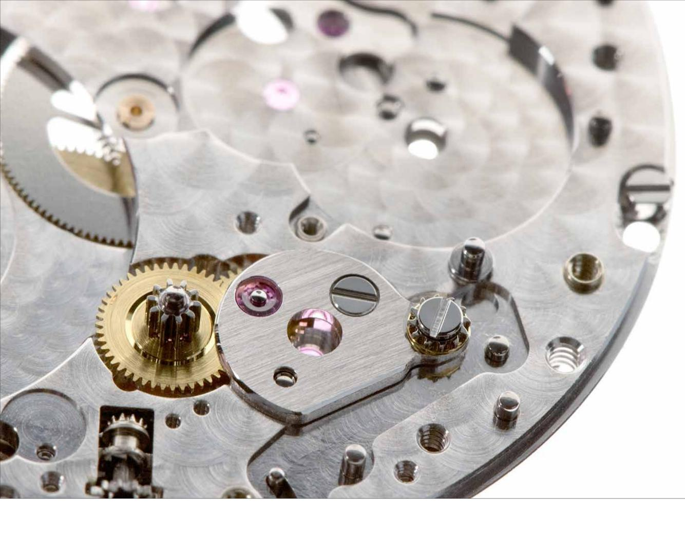
The reverser wheel removed showing the lower bridge holding the Pelton pinion and forming the bearing plate for the first of two wheels continuing to transfer the energy from the rotor to the mainspring.
